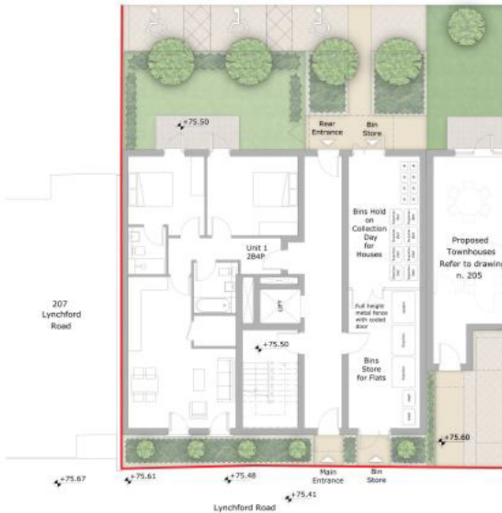
Ground floor plans – Apartment Building (A)
